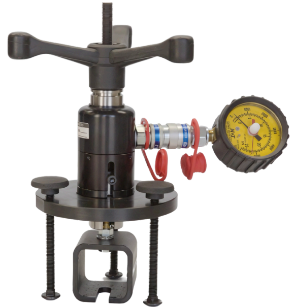
Pullqit™ Anchor Test System with wedge anchor style adapter
